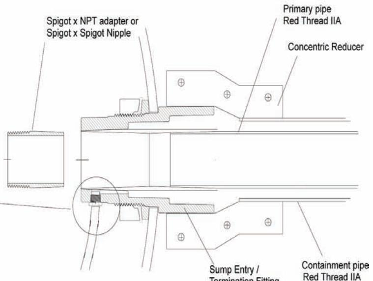
Use concentric reducer to connect the sump entry/termination fitting to secondary containment pipe; DO NOT USE clamshell termination fittings with this style fitting.
