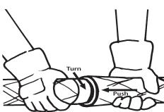
For 1"-2" diameter pipe, insert the spigot into the bell until the tapered surfaces touch. Then while pushing, turn the joint until it locks tight. Normally, one half to a full turn is needed. Hold in locked position until excess adhesive squeezes out.
