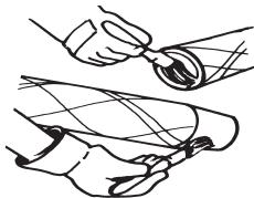
**Note:** Completely coat both bonding surfaces of the joint and remove any loose paint brush bristles in the adhesive.
